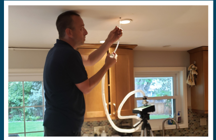
Wall Cavity Sampling
